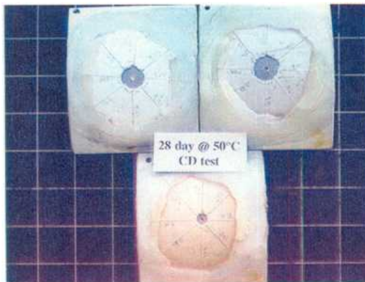
Figure 8: 28 day @ 50°C Cathodic Disbondment Test Panels
