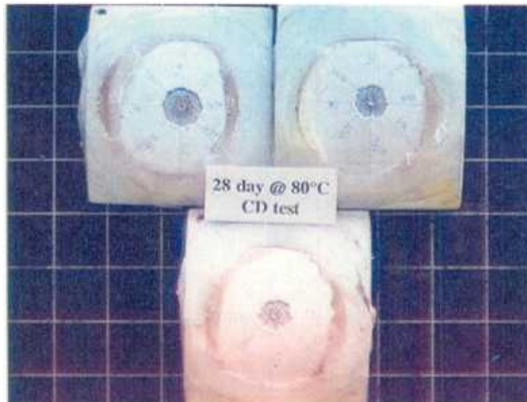
Figure 10: 28 day @ 80°C Cathodic Disbondment Test Panels
