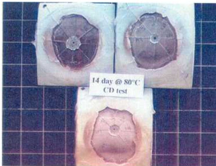
Figure 6: 14 day @ 80°C Cathodic Disbondment Test Panels
