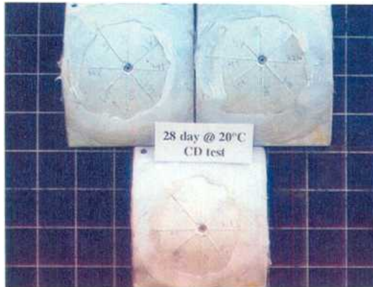
Figure 7: 28 day @ 20°C Cathodic Disbondment Test Panels
