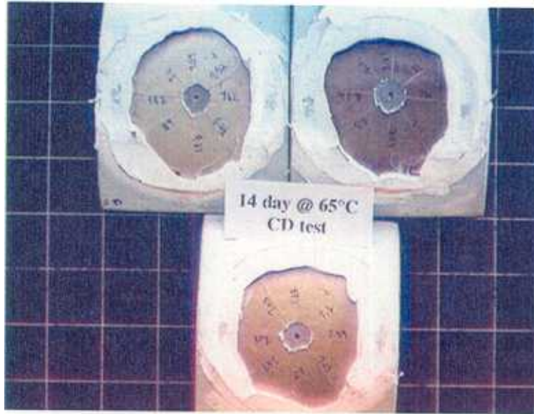
Figure 5: 14 day @ 65°C Cathodic Disbondment Test Panels
